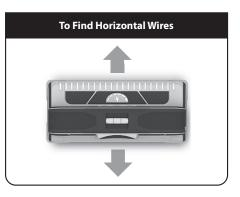
The ProSensor 7000+ uses Active Learning Technology™. To best detect the presence of live electrical wires, slowly scan in both directions, passing over the same location multiple times, for a more accurate reading
